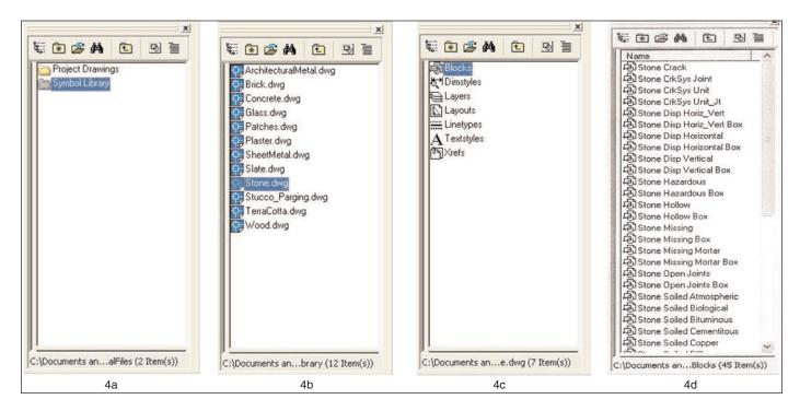
Fig. 4. Double-tapping the Symbol Library folder in Figure 4a brings up the list of block-library drawings shown in Figure 4b. Double-tapping Stone.dwg in Figure 4b generates a list of content types available from that drawing, shown in Figure 4c. Double-tapping Blocks in Figure 4c produces a list of all the blocks in the stone block library, shown in Figure 4d. The blocks in Figure 4d can be dragged and dropped into the open drawing.
