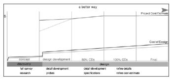
Fig. 2. Cost vs. time graph for a project for which a full survey is completed during discovery.
